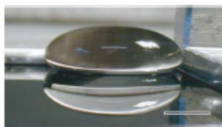
Leidenfrost water drop levitating on a silicon wafer at 200^\circ\text{C}
