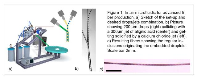
To date, it has been possible to suspend and print cells in the form of regular droplets. The quick sol-gel transition has also been successfully achieved while employing ethanol in the calcium chloride jet. Preliminary results show that ethanol removal, without further modification of the formulations, leads to rather wet, irregular and not very robust hydrogel fibers. Thus, the main challenge of this project is to adapt the sol-gel process to improve its compatibility with living cells.
