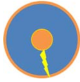
Fig. 4 LG-fault in a cable section.
