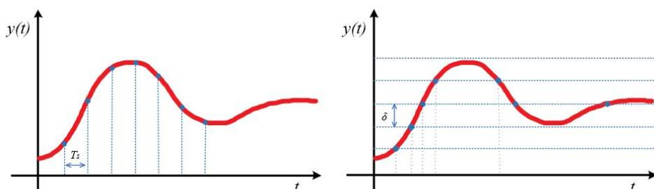
Figure 1: Timer-triggering and Event-triggering approach.
