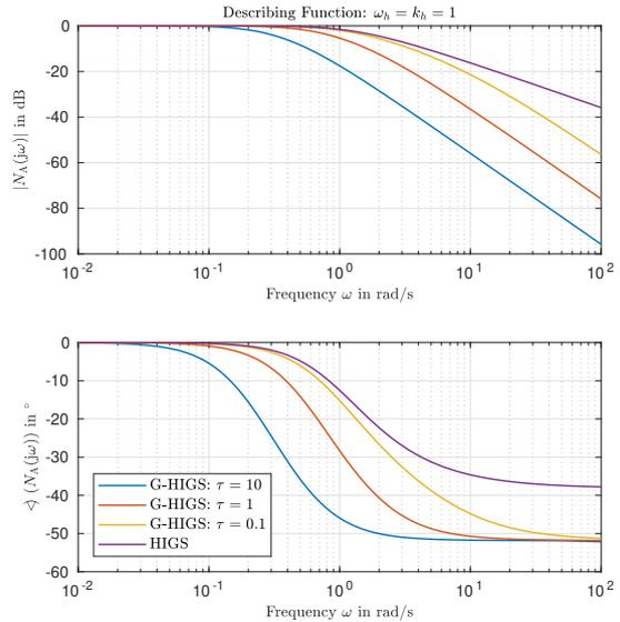
Fig. 2: Amplitude- and phase response of different describing functions.
