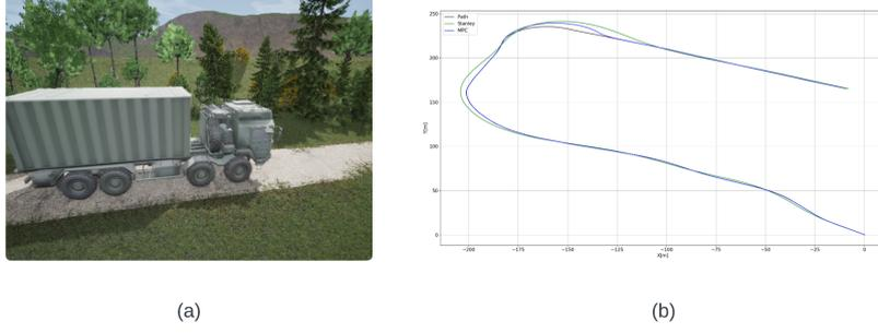
Figure 1: (a) Image of the truck in simulation (b) Comparison of path following between MPC and Stanley controller.
