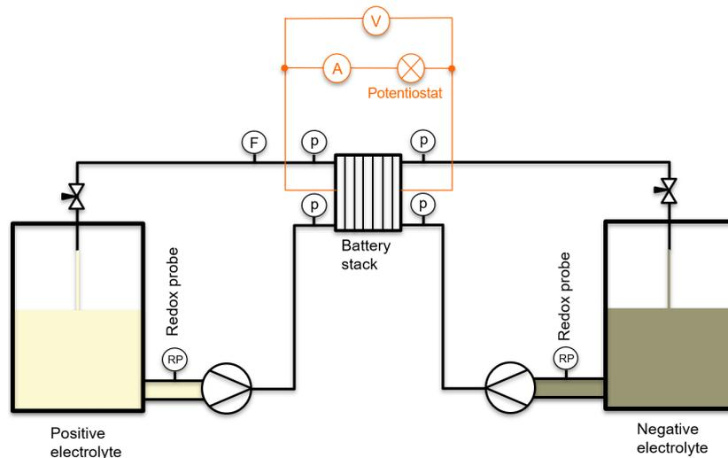
Figure 1: Process diagram of the research demonstrator
