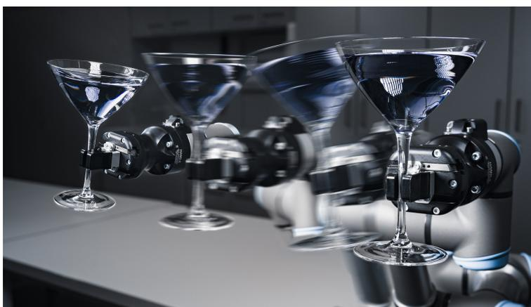
Figure 1: Fast non-sloshing rest-to-rest maneuver with a challenging cocktail glass shape
