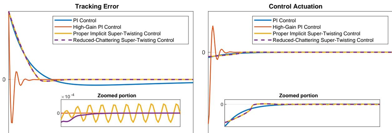
Figure 1: Control of an integrator with a first-order lag-element as unmodeled dynamic.
