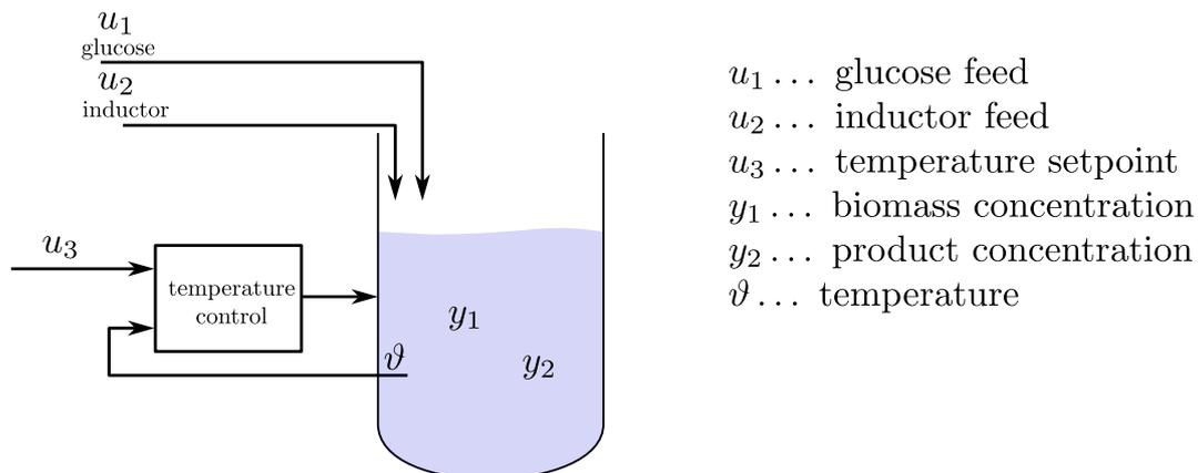
Figure 1: Sketch of a fed-batch reactor.
