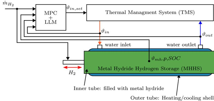
Figure 1: Block diagram of the control strategy.
