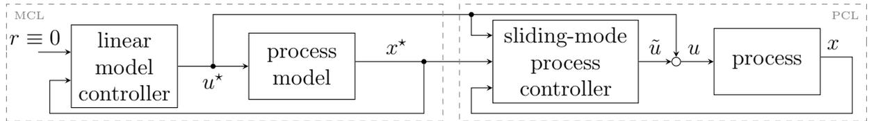
**Figure 1:** Model-following control (MFC) block diagram with sliding-mode process controller.
