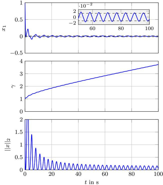
Fig. 6. Simulation of the closed loop system: The upper plot shows the states  $x_1$  and  $x_2$  of the system. The lower plot shows the temporal evolution of the adaptation variable  $\gamma$ , discretized with Euler-forward
