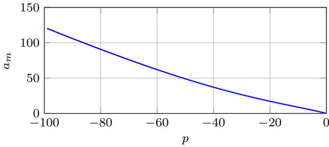
Fig. 3. Relation of the maximum adaptation speed  $\alpha_m$  to controller gain  $p$
