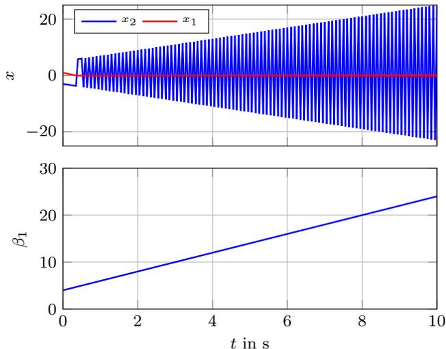
Fig. 1. Simulation of the closed loop system: The upper plot shows the states  $x_1$  and  $x_2$  of the system. The lower plot shows the temporal evolution of the adaptation variable  $\gamma$
