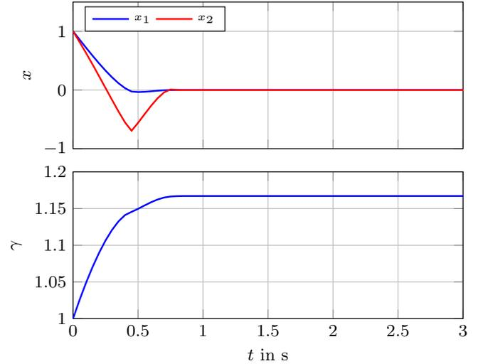
Fig. 4. Simulation of the closed loop system: The upper plot shows the states  $x_1$  and  $x_2$  of the system. The lower plot shows the temporal evolution of the adaptation variable  $\gamma$ , discretized with the Matching-approach
