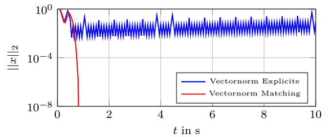
Fig. 5. Comparison of Matching- and Euler-forward approach: The vector norm of  $x_1$  and  $x_2$  shows a discretization chattering which increases in amplitude with the Euler-forward discretization whereas the Matching-approach allows for a smooth transition to zero of the vector norm.
