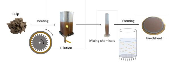
**Scheme of experiments:** Preparation of paper in the laboratory to investigate the effect of cationic starch-soy protein hybrid on paper performance
