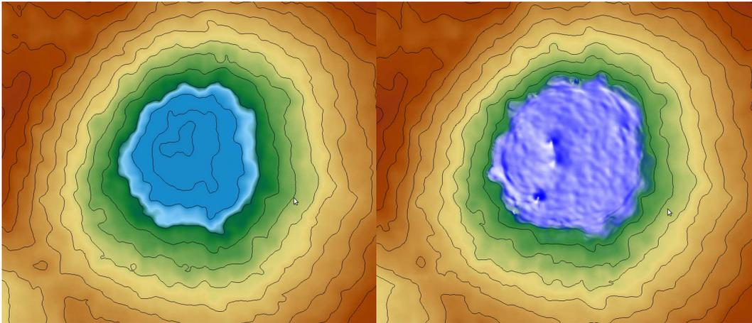
Figure 3: Sand surface based on different altitude without liquid (the left panel), liquid injection in the region of lower altitude (the right panel).
