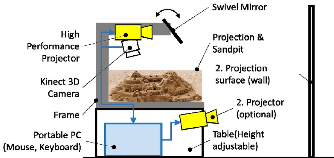
Figure 1: Planned virtual sand box (front view).
