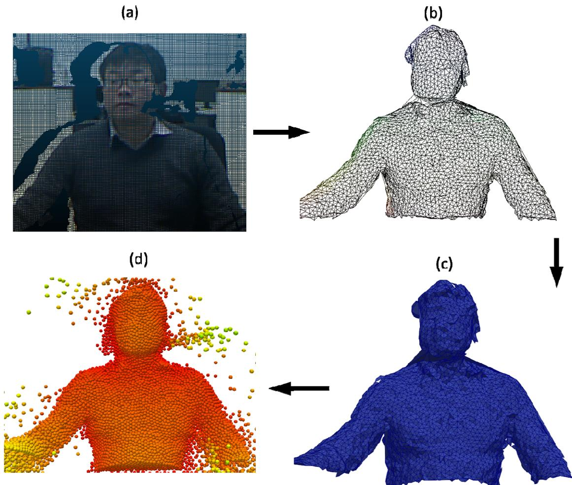
Figure 4: Conversion of the output of the Kinect camera to be fed into the particle simulator LIGGGHT® (i.e., a: camera output, b,c: conversion of the geometry to vtk and stl format, d: filling of the geometry with particles).
