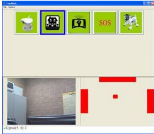
Figure 2: Appearance of the feedback screen. The Feedback application has been instructed to divide the window into three panels. In the top panel, the available selections (commands) appear as icons. In the bottom right panel, a feedback stimulus by the BCI. In the bottom left panel, the Feedback module displays the video stream.
