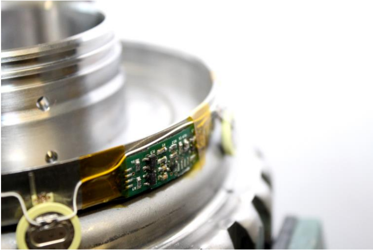
battery powered liquid/gas sensor on rotating gear
