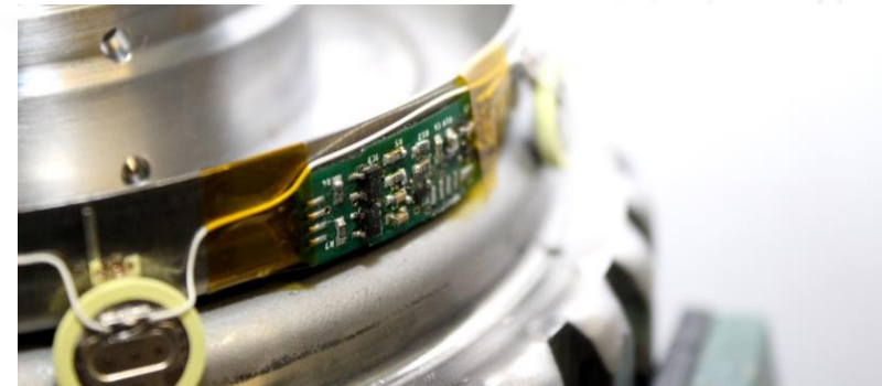
Wireless & battery powered sensor node One week continuous operation
