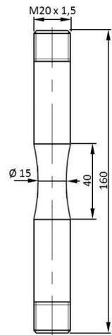
Figure 1: Tensile test specimen for the BETA 250-5 machine.
