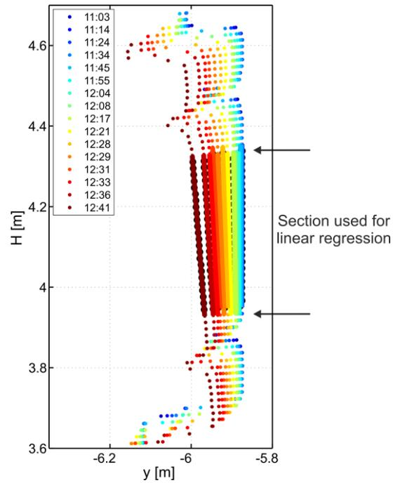
Figure 14. Scanning points on steel traverse from 11:03 to 12:41
