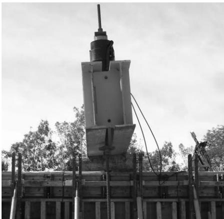
Figure 13. Deformations of steel traverse at 650kN/m<sup>2</sup>
