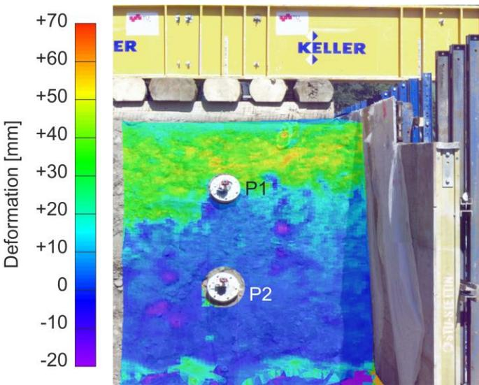
Figure 16. Deformations calculated from point cloud data
