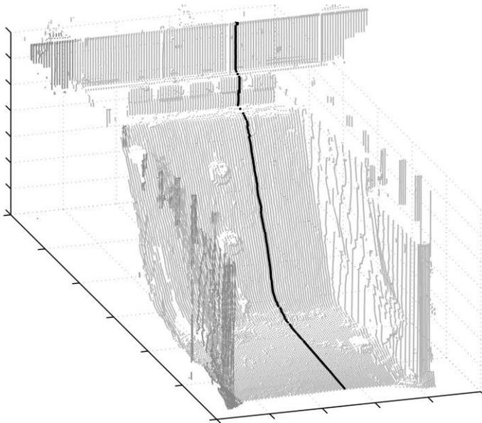
Figure 10. Point cloud of dam surface and single scan line for detailed analysis
