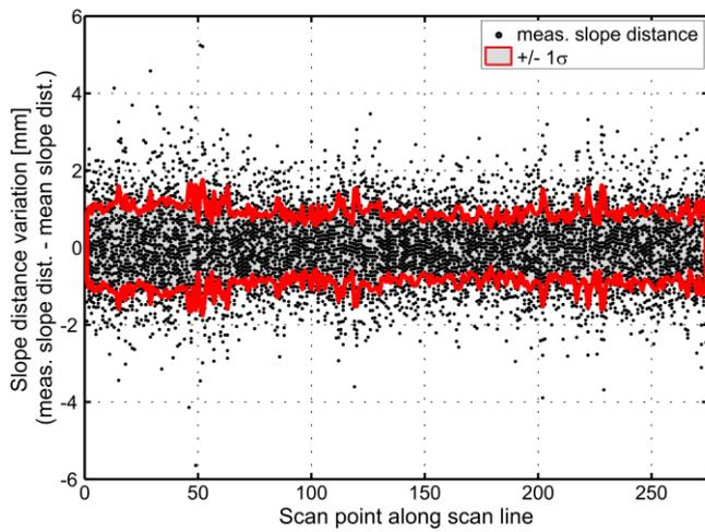
Figure 12. Precision of the observed slope distances
