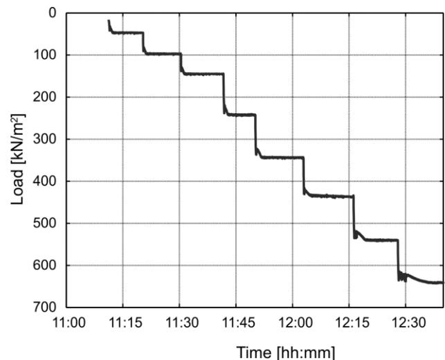
Figure 7. Stepwise increase of load on August 30<sup>th</sup>, 2012
