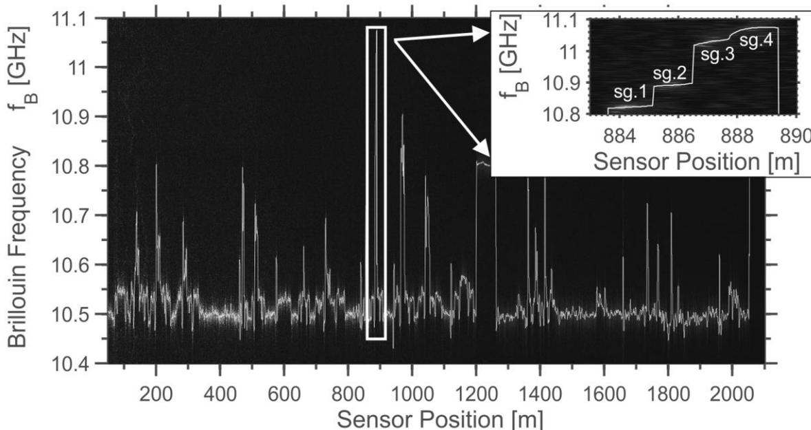
Figure 6. Measurement result of the 2km sensing cable
