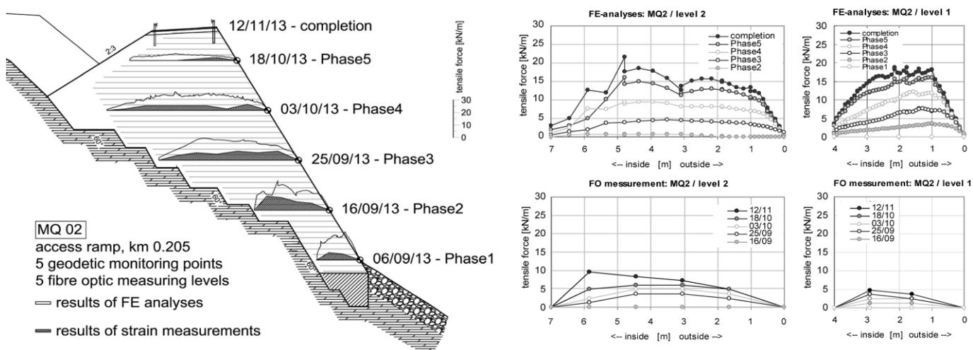
Figure 8. Cross section CS2 at the reinforced earth structure of the access ramp; geogrid tensile forces predicted using finite element (FE) analyses (top right) and derived from fiber optic strain measurements (bottom right)
