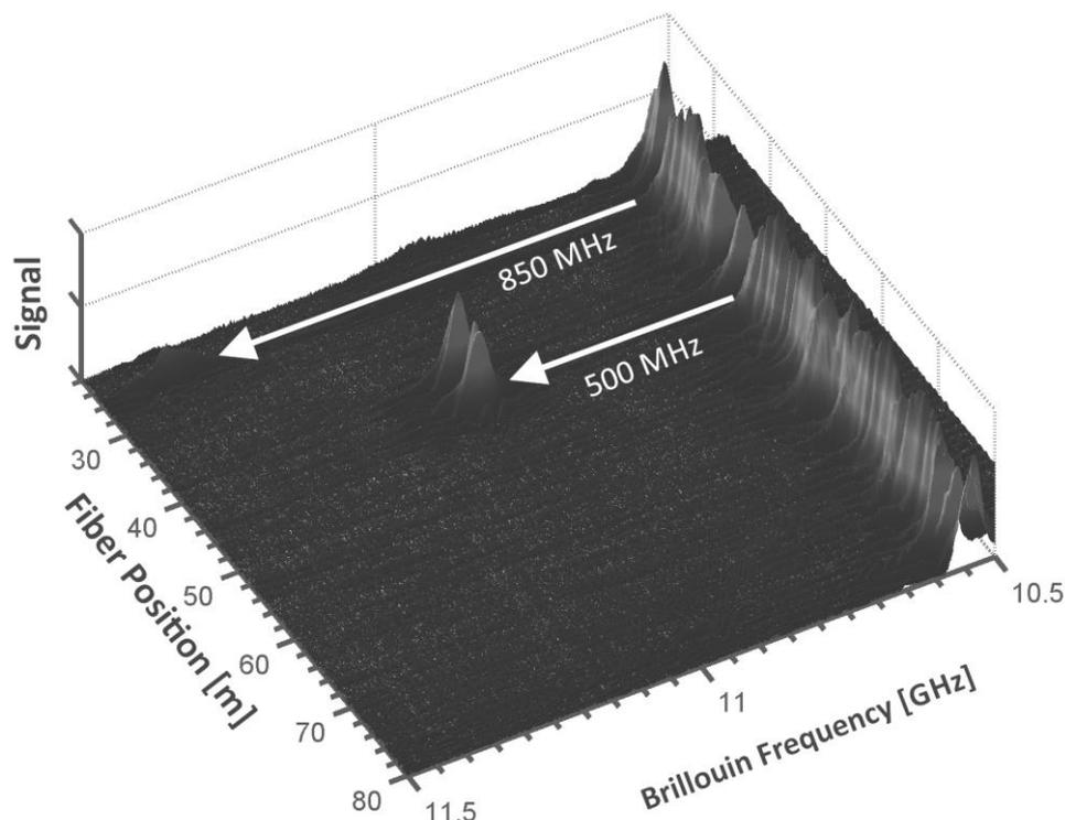
Figure 2. Brillouin frequency spectrum along a sensing fiber
