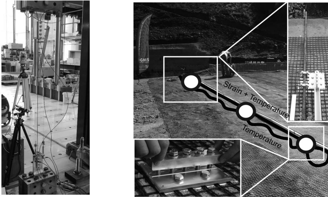
Figure 5. Strain coefficient determination in the laboratory (left); sensor installation on the construction site (right)
