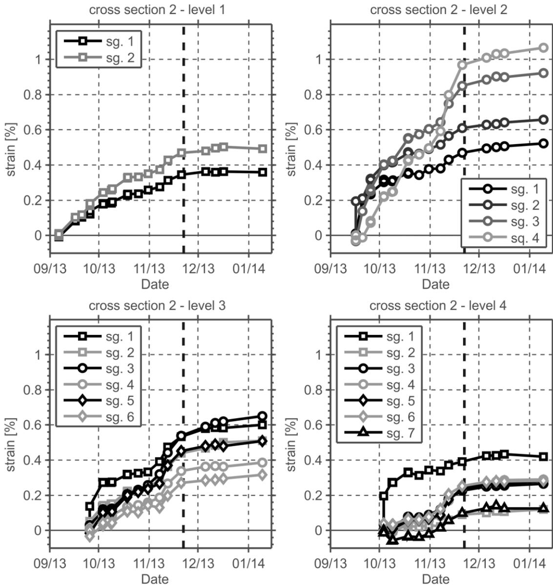
Figure 7. Strain development of the segments (sg.) in the levels 1 to 4 in cross section CS2; the bold dashed line marks the end of the construction works
