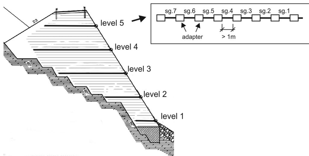
Figure 4. Cross section CS2 with monitoring levels and segments (sg.)
