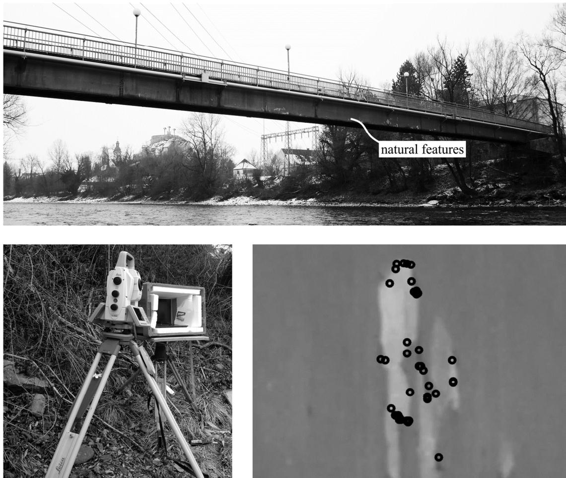
Figure 1. Exemplary setup for the monitoring of bridge vibrations with an IATS (bottom left) and observed image data with automatically detected features of the structure (bottom right).
