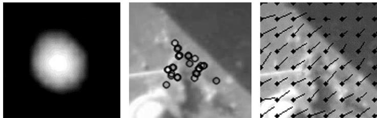
Figure 6. Different processing methods for computing pixel movements from natural targets. Left: template matching with correlation map. Middle: feature matching with detected keypoints. Right: optical flow with movements of selected pixel.
