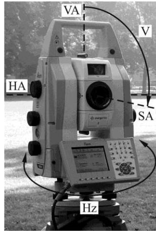
Figure 1. MS50 total station from Leica Geosystems with camera located in the optical path of the telescope. The telescope axis coincides with the sighting axis (SA) of the total station. The telescope can be rotated about the vertical axis (VA) and the horizontal axis (HA). The measured quantities are the horizontal (Hz) and the vertical (V) angles and the distance (measured along SA) to a target.
