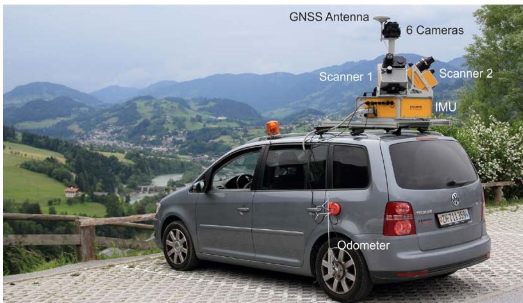
Fig. 3 Mobile mapping system for monitoring retaining walls
