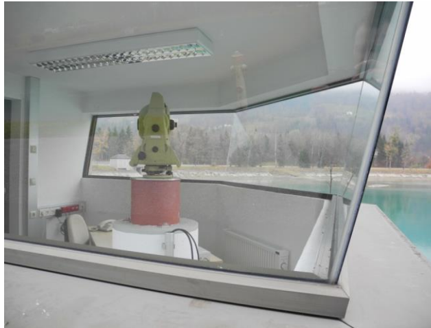
Figure 2: RTS measurement setup for the monitoring of a water dam
