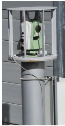
Figure 5: RTS monitoring setup without windows (left) and impact of temperature changes on the tilt sensor of different RTS (right)
