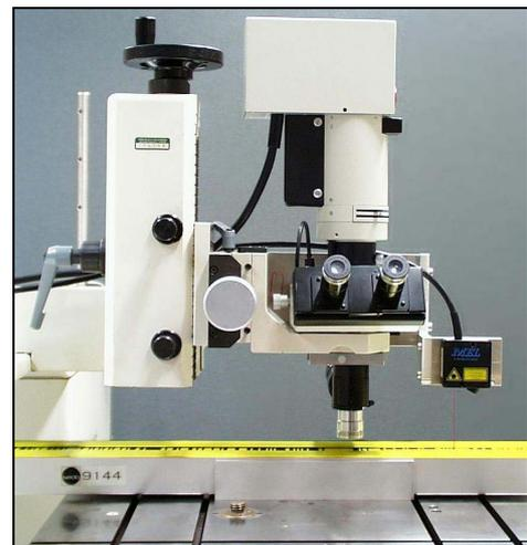
Figure 3: Electro-optical microscope for edge detection
