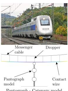
Pantograph - Catenary model
