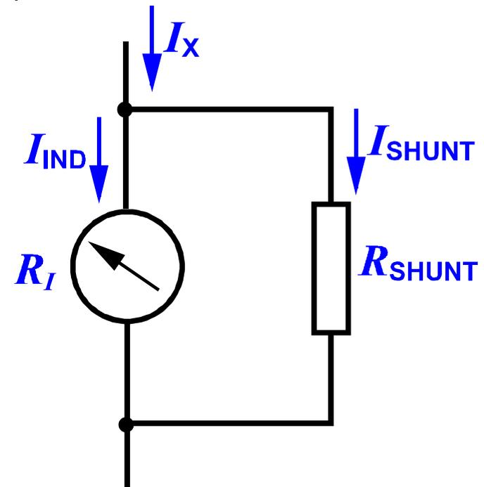
$$I_{IND} = \frac{R_{SHUNT} + R_I}{R_I} \cdot I_x \quad \Rightarrow \quad I_x = \left( 1 + \frac{R_I}{R_{SHUNT}} \right) \cdot I_{IND}$$
