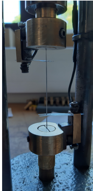
Figure 2.2.: Wire placed in the sample holder with attached voltage knives.
