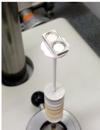
Figure 3: The DSC 404 probe holder with DSC- $c_p$  head
