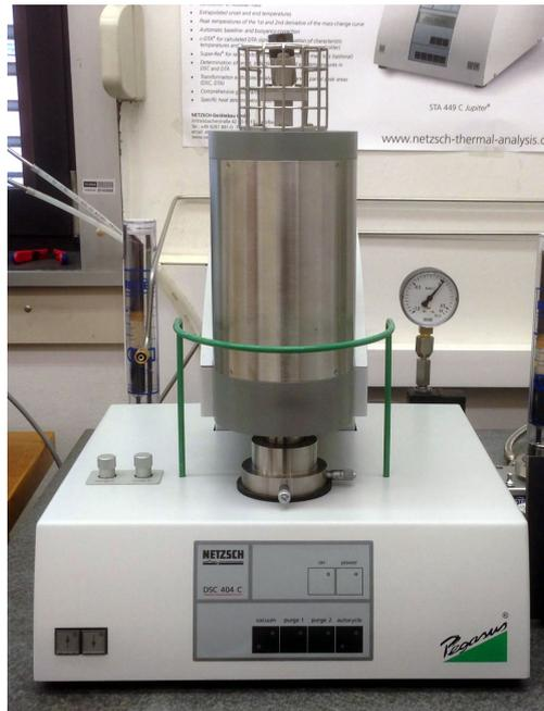
Figure 4: The Netzsch DSC 404 C high temperature heat flux calorimeter
