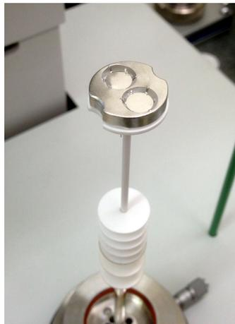
Figure 5: The DSC 404 C probe holder with high accuracy DSC- $c_p$  head
