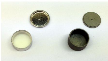
Figure 7: Pt crucible with  $\text{Al}_2\text{O}_3$  insert and graphite crucible, including lids
