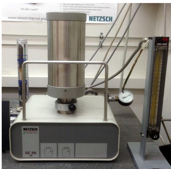
Figure 2: The Netzsch DSC 404 high temperature heat flux calorimeter
