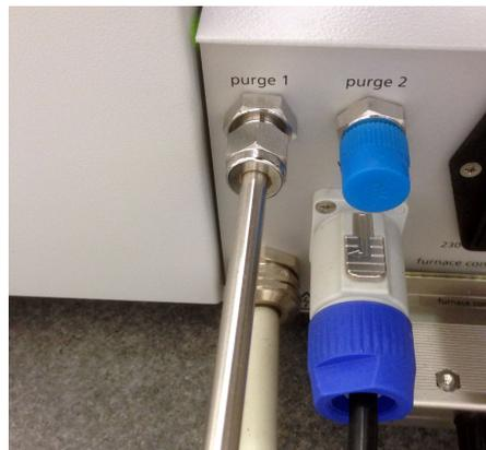
Figure 41: DSC 404 C showing the inlet valves and the connecting purge gas line to the measuring chamber
