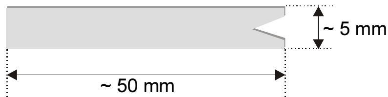
Fig. 15: Schematic drawing of the knife-edge probes. (One of the probes can be seen in Fig. 16a)
