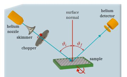
A helium beam is produced in a source chamber, before being scattered from the sample. The scattered beam is monitored with a mass-spectrometer detector. Momentum transfer occurs due to scattering of the He beam from the crystal, at a certain incident angle  $\vartheta_i$ . Energy resolution is optionally added by chopping the He beam with a chopper and measuring the time-of-flight.
