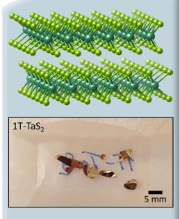
Drawing of the  $TaS_2$  crystal structure (top panel), showing the layered (2D) arrangement of the atoms and a photo of the grown samples (bottom).
