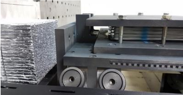
Figure 1: Cells mounted on testbed construction © SafeBattery
