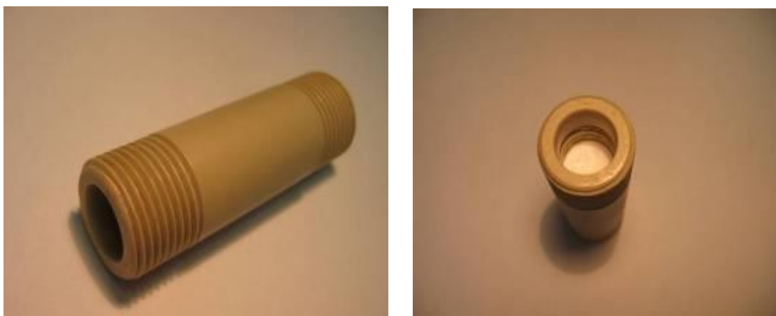
Figure 6. Column for flow-through set-up with the polyHIPE inside
