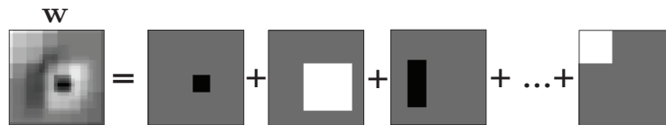
Fig. 1. To compute our binary descriptor, we learn from a training set of corresponding image patches several discriminative linear projections that can be computed from a linear combination of a few simple filters. For the example of this figure, we used rectangular filters that can be computed efficiently with integral images, but we also consider box and Gaussian filters which are also efficient to compute. This approach enables us to build our binary descriptor fast while leveraging on training data.
