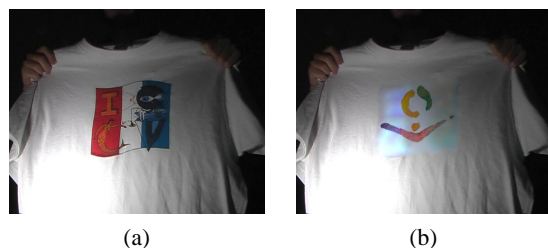
Figure 3: (a) original image. (b) The ISMAR logo replaces the shirt print. Recovering white is hard in this image since the model has large single-colored areas, making light evaluation difficult.
