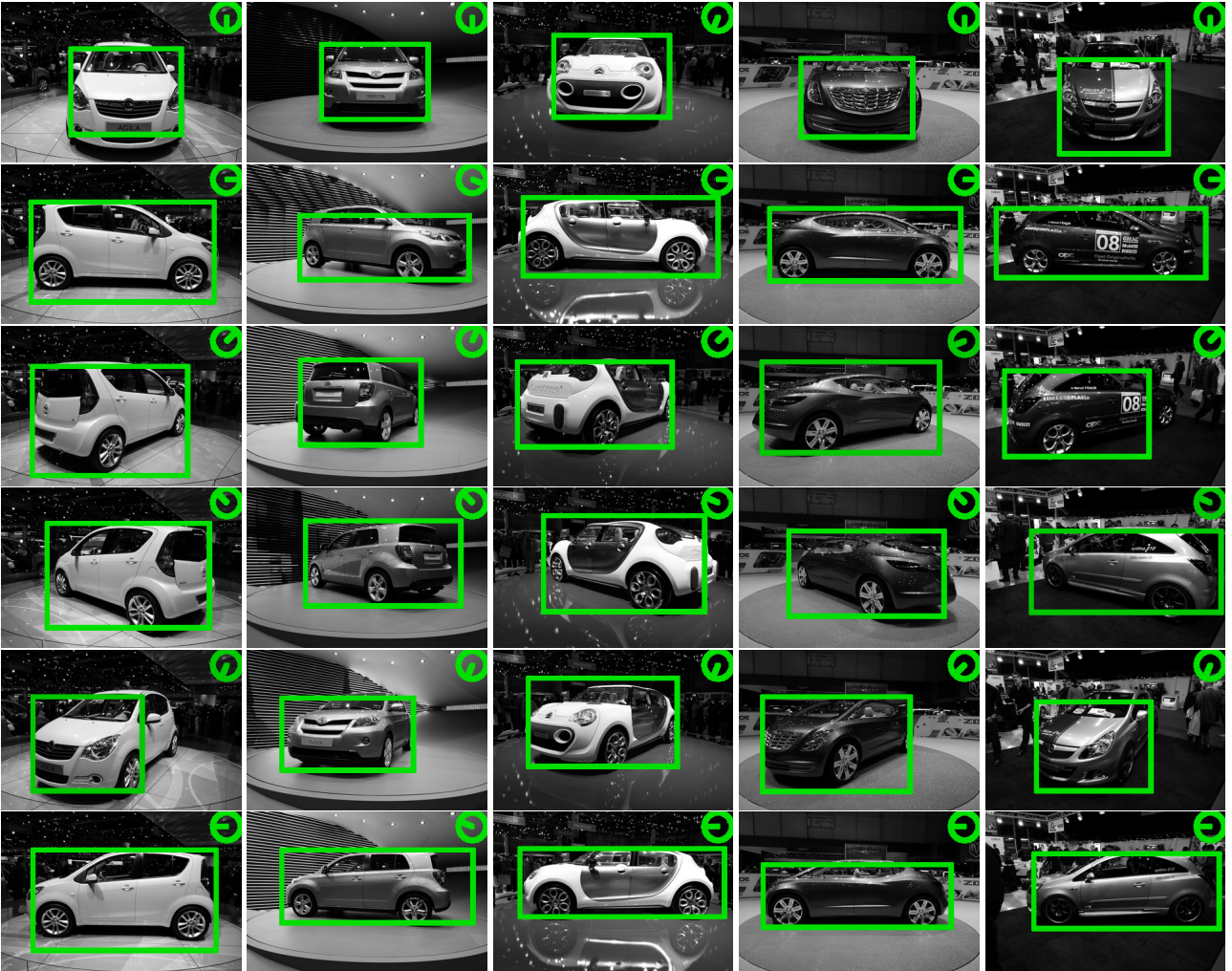
Figure 1. Sample detections from the test set. The green rectangle depicts the recovered bounding box and the estimated viewpoint is indicated inside the green circle at the top-right corner. A front facing car is indicated by a downward pointing line. Despite the challenging lighting conditions and changing backgrounds our approach can correctly localize cars and estimate their pose.
