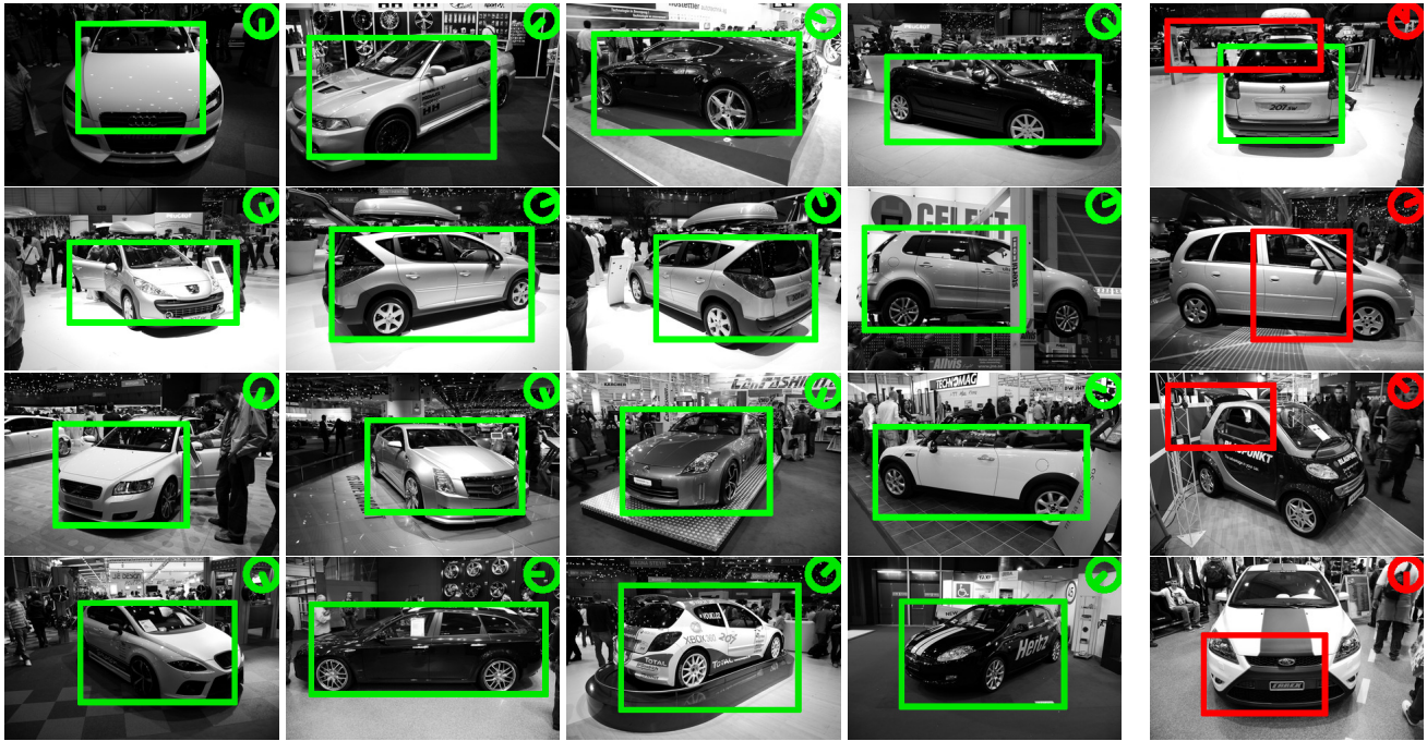
Figure 8. Detections from the car show environment. We show correct detection results except in the last column which contains some false positives.
