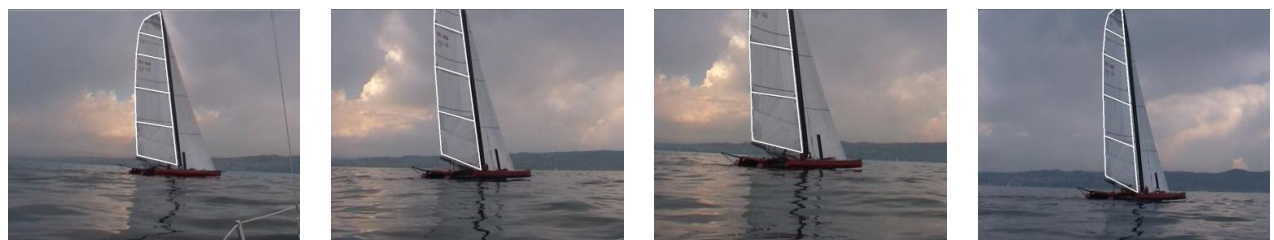
Fig. 14. Detecting a sail. Four frames from a 4000 frame video acquired using a home camcorder during a regatta. Even though the camera jerks, the zoom changes and the lighting conditions are poor, the sail is detected in all frames, such as those shown above, where a sufficient portion of the sail is seen.
