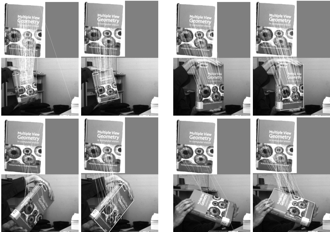
Fig. 16. Comparison with SIFT (left image) and our approach (right image). When there is little distortion, the SIFT approach gives a few more matches, but when too much perspective distorts the object image, it gives only few matches, while our approach is not perturbed.
