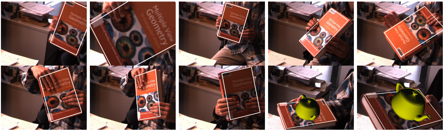
Fig. 1. Detection of a book in a video sequence: As shown by the white outline, the book is detected independently and successfully in all frames at 25Hz in 640 \times 480 images on a standard PC, in spite of partial occlusion, cluttered background, motion blur, large illumination and pose changes. In the last two frames, we add the inevitable virtual teapot to show we also recover 3-D pose. The corresponding video sequence is submitted as supplementary material.
