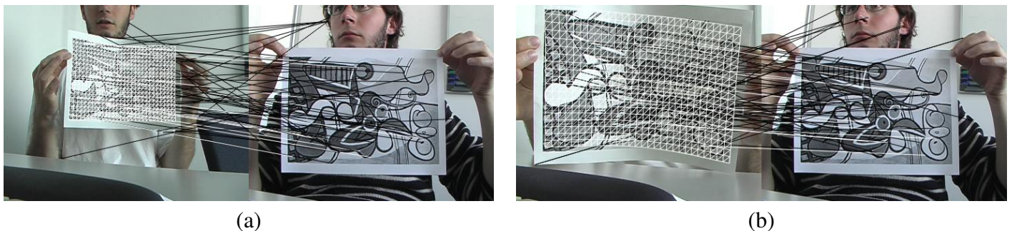
Fig. 19. Detecting a deforming sheet of paper at 10Hz on a 2.8 GHz PC. (a) The left image is the input image in which the sheet of paper is detected and its deformation estimated. The right one is the training image. The lines represent the matches recovered using our method. Black ones correspond to those estimated to be outliers and the white ones to inliers. (b) Same thing for a different input image.
