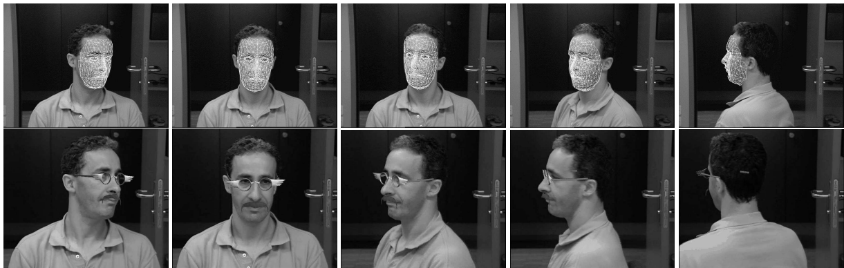
Figure 13. A 3D model of the face is tracked to augment the video sequence by adding glasses and a mustache to the subject.
