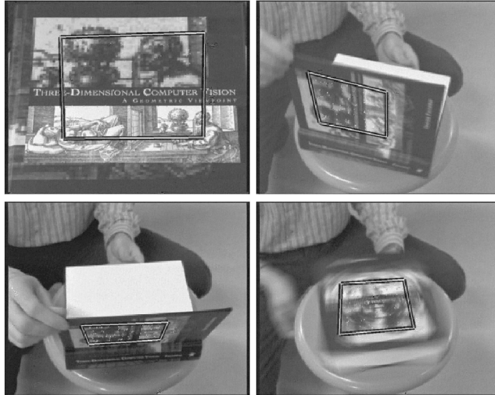
Fig. 4.4 The book cover is modeled as a plane, and tracked using a template matching-based approach. (From [66], figure courtesy of F. Jurie and M. Dhome.)
