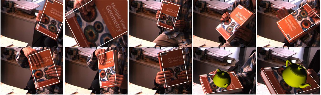
**Figure 1. Detection of a book in a video sequence:** The book is detected independently and successfully in all subsequent frames at 25Hz in  $640 \times 480$  images on a standard PC, in spite of partial occlusion, cluttered background, motion blur, large illumination and pose changes. In the last two frames, we add the inevitable virtual teapot to show we also recover 3D pose. A video sequence is available at <http://cvlab.epfl.ch/research/augm/detect.html>
