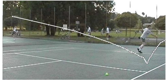
Figure 7: A recovered trajectory from a monocular sequence. Tracking is not lost after the ball has bounced.
