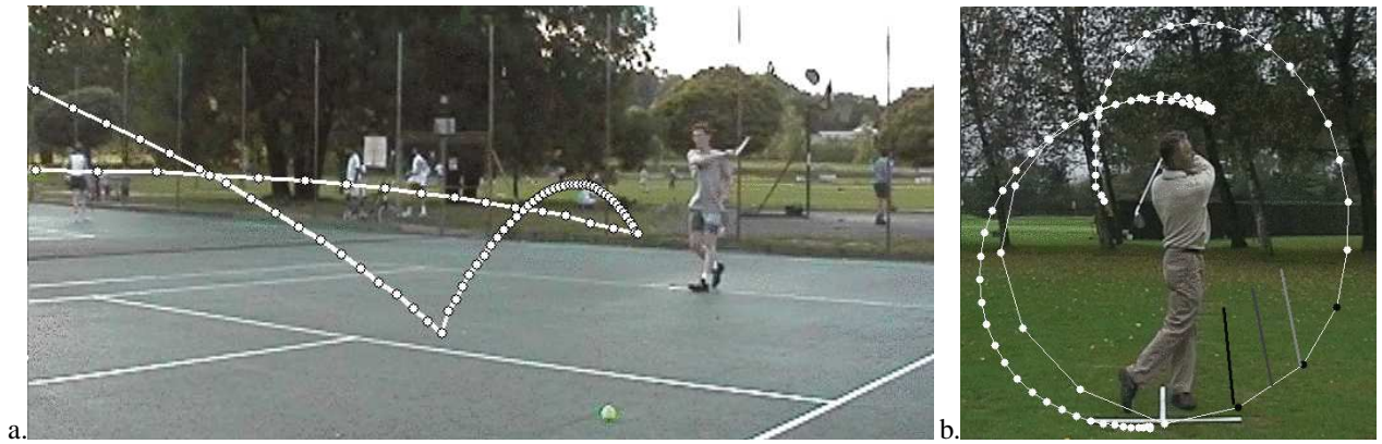
Figure 1: Ball and golf club tracking with our method: (a) the ball tracking is performed without any manual initialization and is not perturbed by motion discontinuities which tend to break Kalman style approaches; (b) the golf club tracking is unperturbed by the mis-detections (corresponding to black disks) and the false-alarms, intentionally added to try to distract the tracker.
