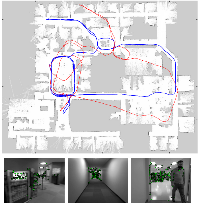
Fig. 1. Top: Skeleton map constructed online from just stereo images, registered against a laser map for reference. Red is visual odometry, blue is corrected by loop closure from visual place recognition. Tick marks at sides of map are 10m intervals. Bottom shows typical views, with blurring, clutter, people, and blank walls.
