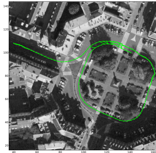
Fig. 8. Versailles Rond sequence of 700 video frames taken from a moving vehicle, 1m baseline, narrow FOV. (Dataset courtesy of Andrew Comport [10]) Top: matched loop closure frames. Bottom: top-down view of trajectory superimposed on satellite image.
