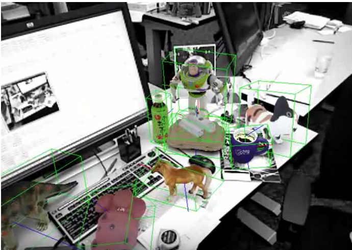
Fig. 1. Several 3D objects are simultaneously detected with our method under different poses on cluttered background with partial occlusion and illumination changes. Each detected object is augmented with its 3D model, its 3D bounding box and its coordinate systems. For better visibility, the background is kept in gray and only detected objects are in color.
