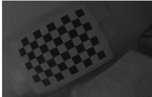
Figure 3: Example for an image used in calibration of the webcams.
