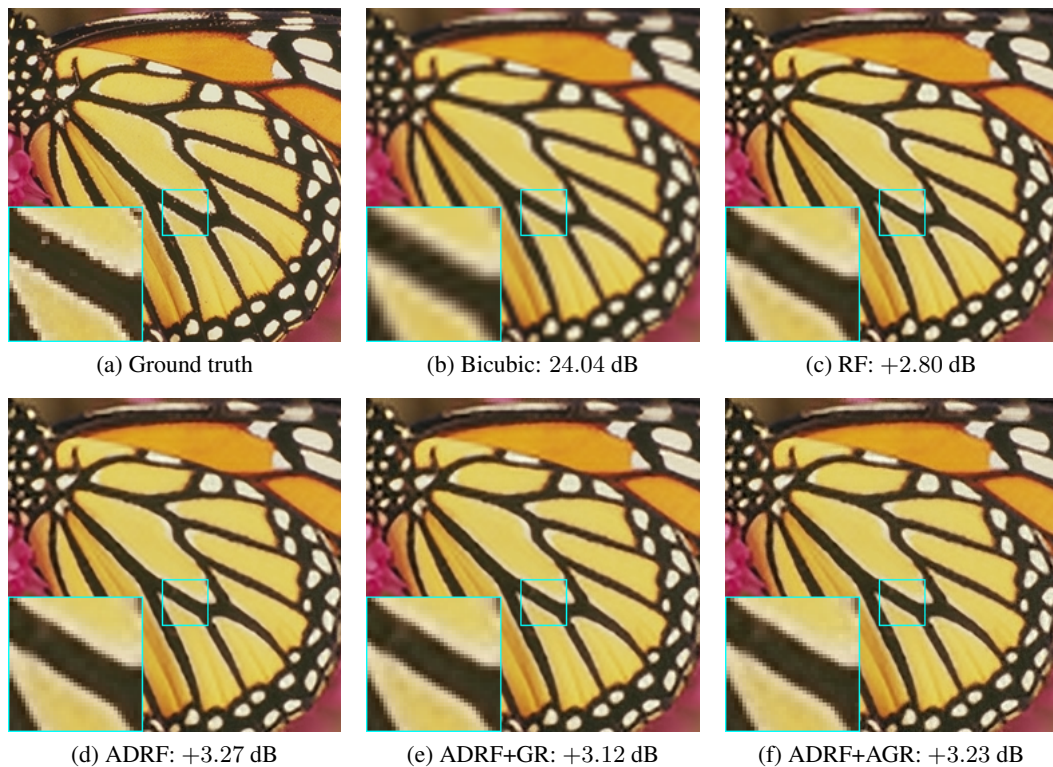
Figure 3: Qualitative SR results for butterfly from Set5 [3] using an upscaling factor of 3. We report the PSNR for the bicubic upscaled image and the gain for different RF approaches. While all of these methods achieve a similar level of visual quality, the size of the used models differs significantly (see Table 2).
