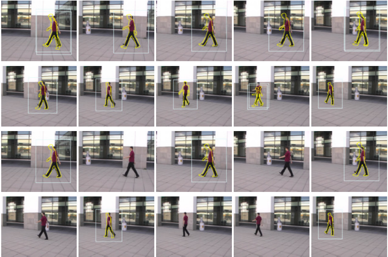
Figure 9. Filtering silhouettes with temporal consistency on an outdoor sequence acquired by a moving camera. First two rows: Detection hypotheses. Third and fourth row: Detections after filtering out the detection hypotheses that do not lie on the recovered most probable trajectory.
