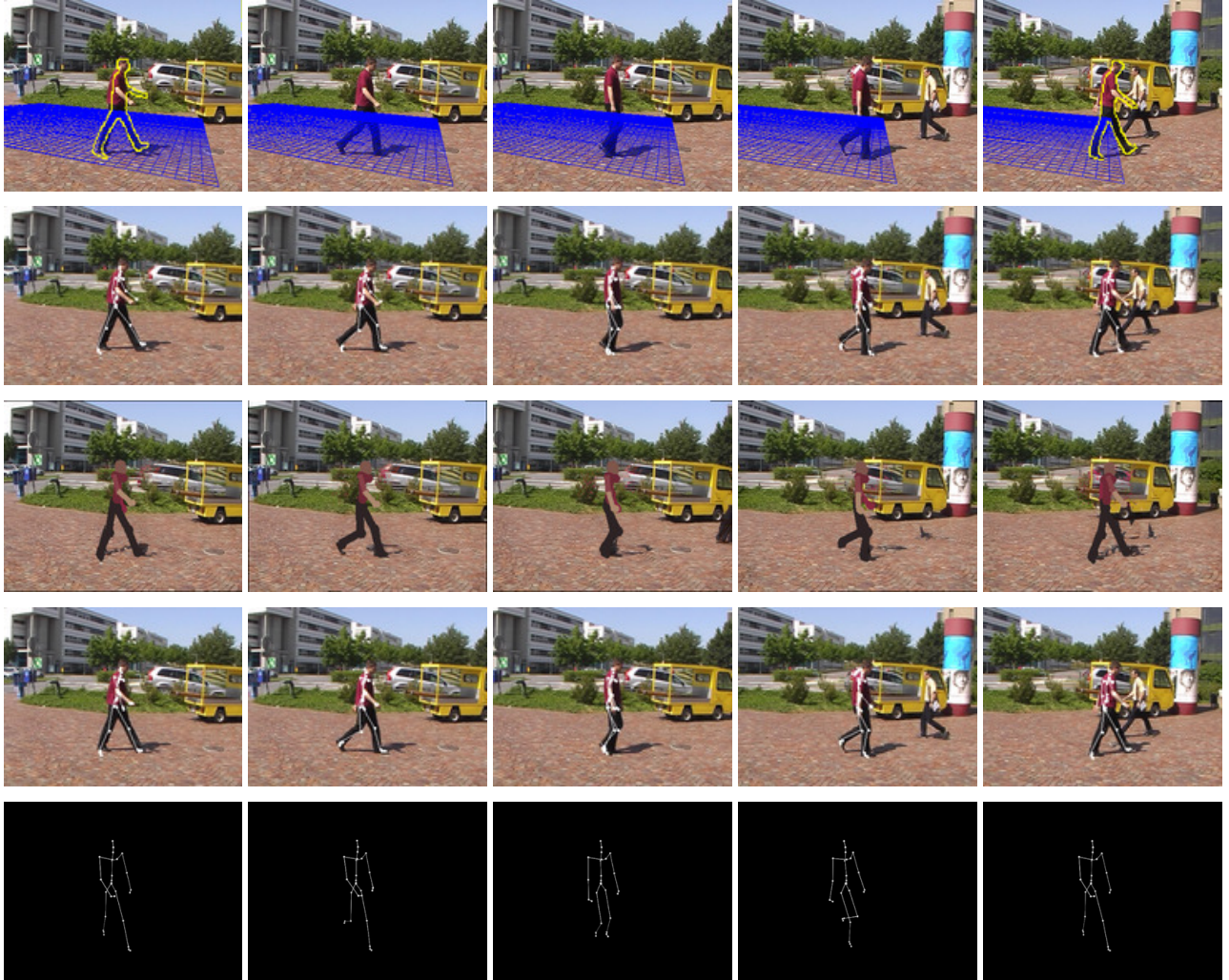
Figure 1. Our approach. First row: Input sequence acquired using a moving camera with silhouettes detected at the beginning and the end of the walking cycle. The projection of the ground plane is overlaid as a blue grid. Second row: Projections of the 3-D poses inferred from the two detections. Third row: Synthesized images that are most similar to the input: Different colors represent different appearance models. Fourth row: Projections of the refined 3-D poses. Fifth row: 3-D poses seen from a different viewpoint.
