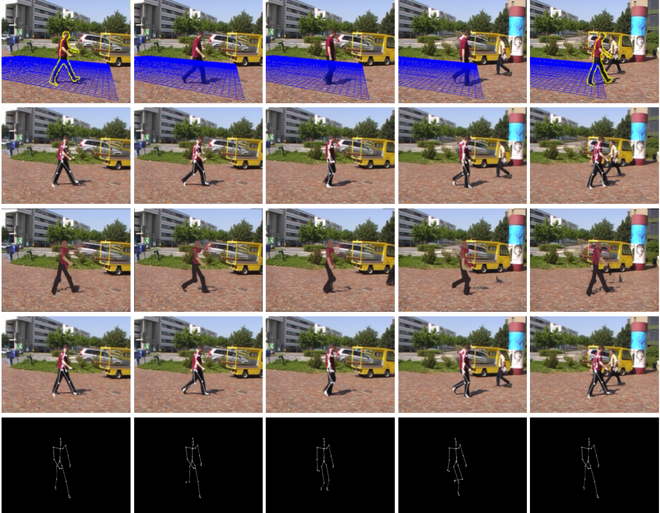
Figure 1. Our approach. First row: Input sequence acquired using a moving camera with silhouettes detected at the beginning and the end of the walking cycle. The projection of the ground plane is overlaid as a blue grid. Second row: Projections of the 3-D poses inferred from the two detections. Third row: Synthesized images that are most similar to the input. Fourth row: Projections of the refined 3-D poses. Fifth row: 3-D poses seen from a different viewpoint.
