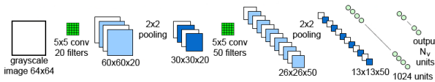
Fig. 5. Architecture of the CNN \text{CNN}_{w}^{\text{cp-pred-}p} predicting the projections of the control points.
