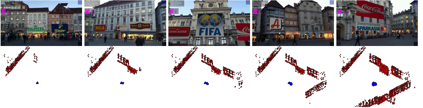
Fig. 11: Top row: Annotation results from a rotation-only sequence. Bottom row: Expanding SLAM map, while the user rotates a handheld device. The map nicely resembles the structure of the surrounding buildings.
