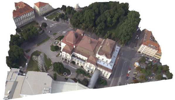
Figure 1: Visualization of a textured 3D reconstruction/DSM derived from our multi-view dense matching method.
