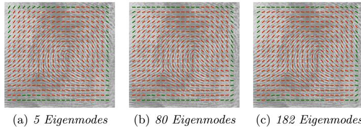
**Fig. 5. Number of Eigenmodes.** In case of too few Eigenmodes (Subfigure 5(a)) the model fails to generalize, especially visible at SPs. The application of a higher number of Eigenmodes allows the model to fit the shown OF more precisely.
