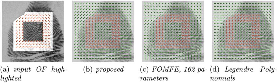
**Fig. 3.** Prediction ability of various methods proposed in literature. Input OF as shown in 3(a). Green color is used to display the interpolated/extrapolated OF. Subfigure 3(b) shows the results of the proposed method. The prediction capability of the FOMFE approach (exactly as in [14]) is shown in image 3(c). Subfigure 3(d) shows results of the approach described in [11] (exactly as described in the paper). Note that the proposed method (Figure 3(b)) generates the most plausible OF.
