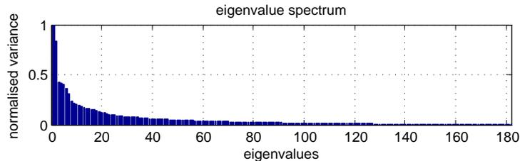
**Fig. 1.** Eigenvalue spectrum of 2000 fingerprint vectors (NIST4 f-prints database). Note how the first 40 eigenvalues correspond to more than 95% of the data’s variance.
