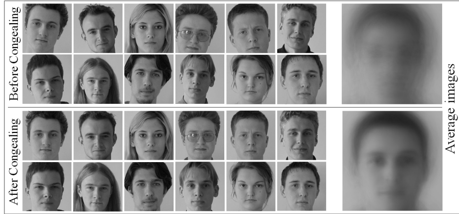
Figure 4. The spatial variation gets removed from the perturbed facial samples by our algorithm. The samples are taken from the CVL database [12].
