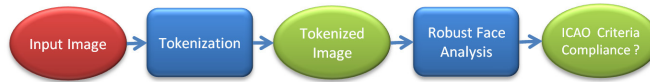
Figure 1: Illustration of the overall image analysis system consisting of normalization ( tokenization ) and compliance analysis.
