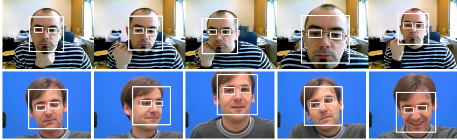
Figure 5: Two examples of input video with detected face and eye positions. Top: natural light, glasses. Bottom: Talking Face video [13].
