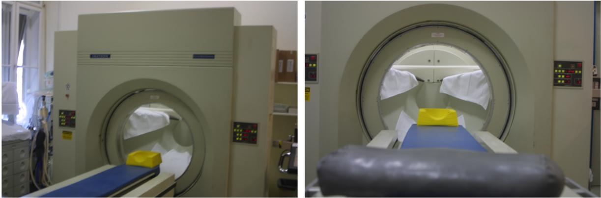
Figure 2.3: The Ultrafast (or Electron Beam) CT scanner located at the Department for Radiology, University Hospital Graz. It is an Imatron Inc. C150 scanner.
