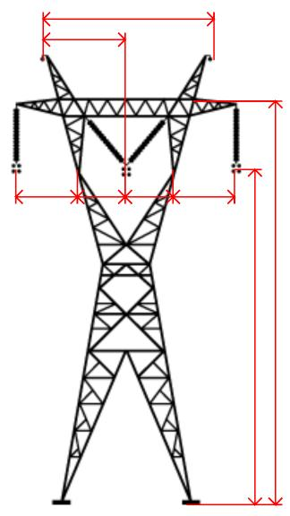
Simplified CAD model of powerpylon. The main measurements are automatically extracted from a 3D Reconstruction. Original image attribution, user: CODinDK; website:https://commons.wikimedia.org.
