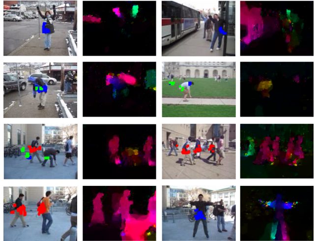
Figure 9. Examples for action detection. First and third column shows detection results of bending (green), walking (red) and waving (blue) action. Corresponding optical flow fields are shown in column two and four.
