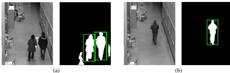
Fig. 3. Motion blobs obtained from background subtraction. Blobs that fulfill the constraints are accepted as positive samples (green bounding boxes).
